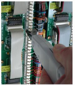
If you wish to cut off the excess wire, remove the clip at the bottom of the tool and allow it to hang free on the string. If you wish to link the wire onto another point, make sure the clip is in place and this will prevent the cutters operating. Please be very careful not to allow the wire clippings to fall into the electronics where they may cause damage.
